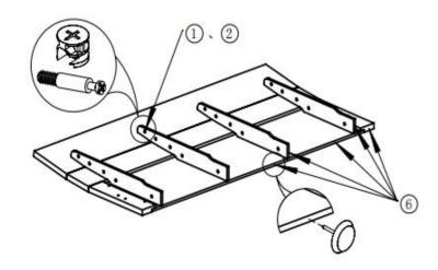
1. The bottom of the1 and 4 installed 6 evenly. The 4 adopts 2 and 1 to connect the 1,2 and 3 respectively.
