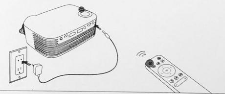
Indicator light will on after plugging in the power cord. Then press the Power button on the rear of projector or on the remote control, it enters into multimedia interfacewithin 2 to 5 seconds.
