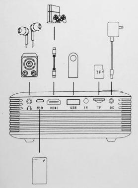
Insert the USB/micro SD card into the accrdingly slot trefer to the picture as below.
