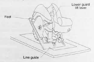
With the blade just clearing the material to be cut, start the motor. Gradually lower the back end of saw using the front end of the foot as the hinge point.
