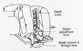
Not more than one tooth length of the blade should extend below the material to be cut, for minimum splintering.
