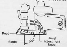
If adjustment is necessary, tilt foot to 45°, tighten bevel adjustment knob and bend "TAB" with an adjustable wrench or pliers.
