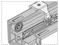
After installing track, try to pull and push for several time to ensure that the rebound divice and rebound stopper match well.
