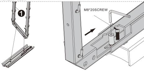
Put the regulating bolt into the rear hole of the main frame.
