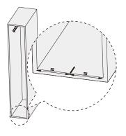
2.2 Drill 6 preliminary holes which diameter is 2.5mm on the bottom panel according to the template.
