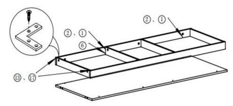
1. a.The 12 use 2,1,6 to connect the 11 and 25, b.The 11 and 25 use 2,1 to connect and fixed 1, c.Use 7 fixed the 3 to the connection of 11,12,25.
