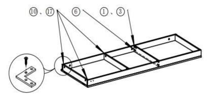
1. a.The 12 use ①,③,⑥ to connect 11 and 21, b.The 11 and 12 use①,③ to connect 1, c.⑩ and ⑰ are fixed at the junction of 12, 11 and 21
