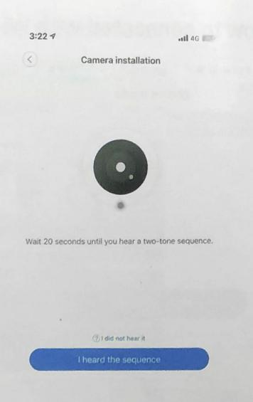
If you don't hear the sequence, please press the "RESET" on the device. Continue for more than 5 seconds, until you heard the sequence, that means the reset is successful.
