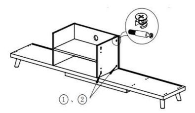
2、 The 4 adopts ① and ② to connect the 2. The 5 is connected to the 2 with ① and ②. The 4 and 5 adopts ① and ② to connect the 6. The 2 and 6 adopts ①,② and ⑤ to connect the 1.
