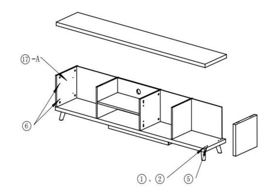
3. Use (6) to install rail (17)-A on the 2 and 3. The 3,9 and 11 adopts (1,2), (5) to connect the 1, and then insert the 10 and 14.
