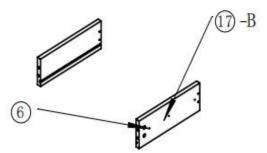
5. Install rail 1-B on the outside of the 16 and 17 by using 6.
