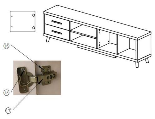
4、 Each 12 using two 13 installed on the corresponding position of the 13. Then uses two 13 and two 14 to connect the 12 and corresponding side plate of the cabinet.
