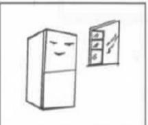
The refrigerator is placed in a well-ventilated indoor place; the ground shall be flat, and sturdy (rotate left or right to adjust the wheel for levelling if unstable).
