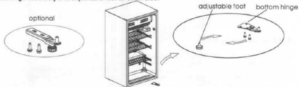
5)put the door on bottom hinge and assemble the upper hinge, upper hinge cover and plastic screw hole caps successively.
