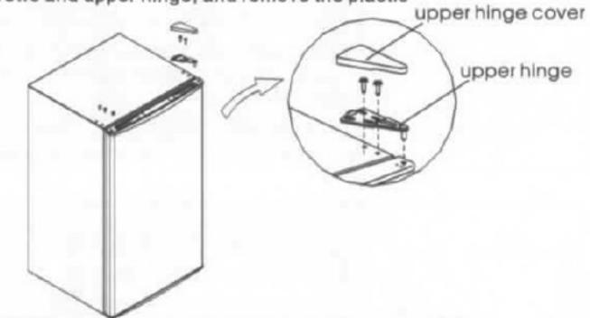
4) dismantle the door and the bottom hinge assembly and adjustable foot, then assemble the bottom hinge assembly and adjustable foot on other side.
