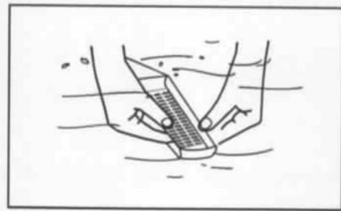
3: Push down the filter screen and insert it into the groove, ensure that it has been installed in place without looseness.
