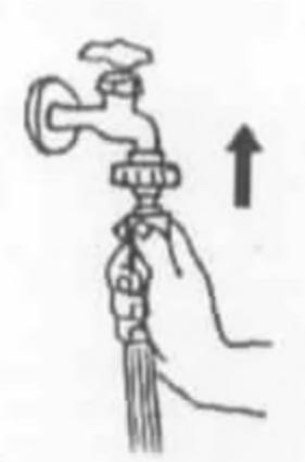
4.2 Switch connector tightly to make rubber tap press tightly on the tap bore until it is completely prevented from water leaking.
