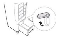
Push the water tank button out to horizontal state√
