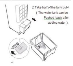
3 Turn the knob off by hand, (According to the 90° counterclockwise) Separate the water tank from the pump module.. (Including the pipe)..
