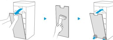
Air outlet grill Open the air outlet grill, vacuum up dust with a vacuum cleaner, and wipe it with a cloth
