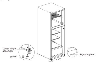
5)Dismantle the limit blocks and screws on the lower cover of both refrigerator door and freezer door, install them on the other side of both doors; then install the sleeve pipe on the upper cover of the refrigerator door on the other side.
