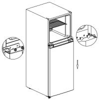
7) Install the freezer door on the middle hinge, and install the upper hinge, hinge cover and hole cover
