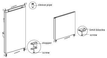
6) Install the Refrigerator compartment door on the lower hinge and then install the middle hinge andhole caps.
