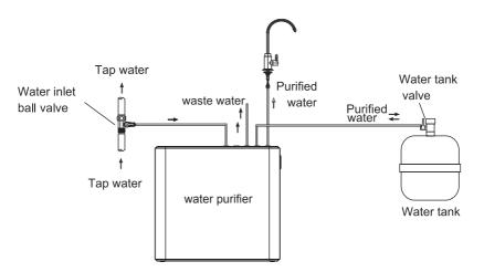
**Remarks:** The unit should always be standing( the top cover should always turn upwards), the unit cant be placed horizontally or tilt to one direction
