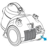
05 Turn on the machine: press the on/off switch pedal, the machine could start working.
