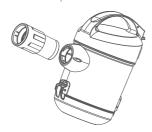
02 Connect the plastic tube to the curves end of the hose.
