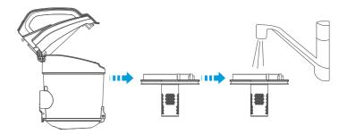
04. Install the filter core: After cleaning, put the filter into the dust cup and notice the direction of the arrow.
