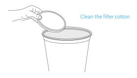
**03.** Remove and clean the filter core:
