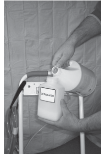
Figure 6: Filling pre-spray bottle with Demon Clean >>>
