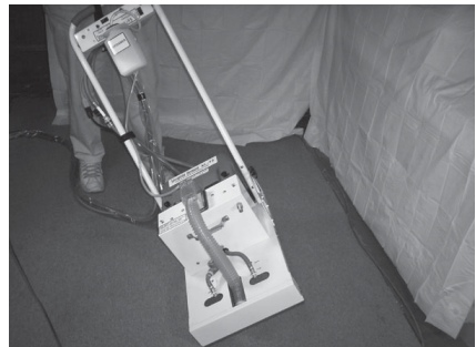
Figure 23: Tilting machine to the right to manually activate discharge pump
