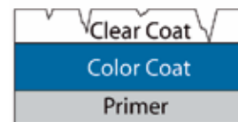
Profile image of paint with various scratches.
