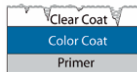
Profile image of paint with scratches in and oxidation and pollutants on the clear coat.
