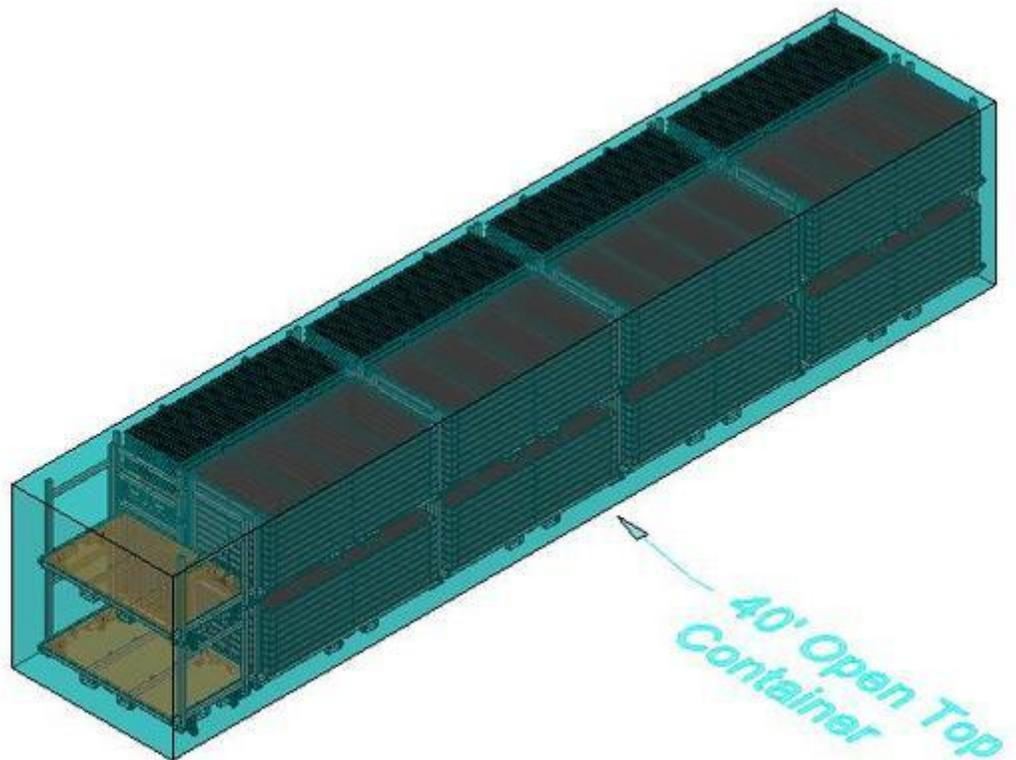
We designed 48" and 41" wide carts ,in order to be able to load side by side in the sea containers that are maxed in width.
