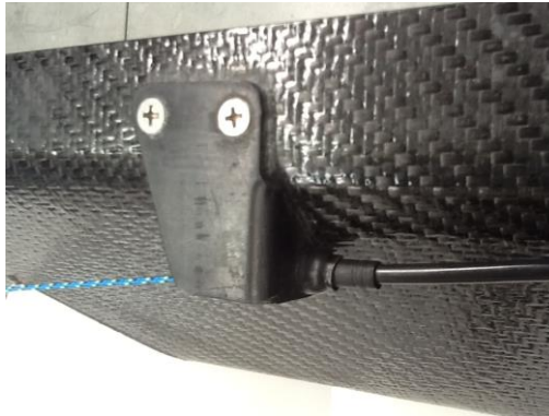
Figure 6 - Outer cable end cap fitting into the Bowden clamp
