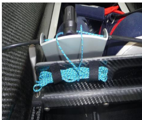
Figure 4 - Correct location and orientation of the Velcro tabs
