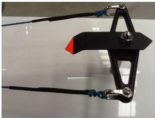
Figure 7 - Spectra cable tied onto the rudder head and finished using the heat shrink
