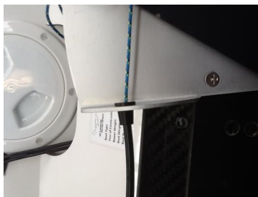
Figure 2 - Outer cable fitting into the steering foot plate
