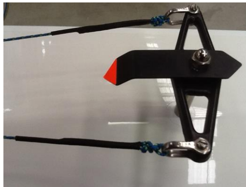
Figure 3 - Spectra cable tied onto the rudder head and finished using the heat shrink
