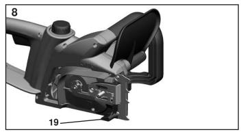
This chainsaw is fitted with a chain catch bolt (19). If the chain breaks when the saw is in operation, the chain bolt will catch the loose chain end and thus prevent injury to the operator's hand.
