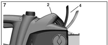
This chainsaw is equipped with a mechanical brake for the chain. In the case of uncontrolled movements, when the tip of the saw blade gets in contact with wood or a solid object, the drive of the chain is immediately
