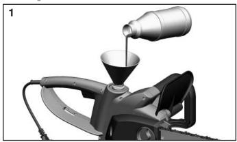
The chainsaw must never be operated without sufficient oil on the chain as this could cause damage to the chain, blade or motor. No claims for guarantee can be accepted if damage occurs when the device is being operated without chain oil.
