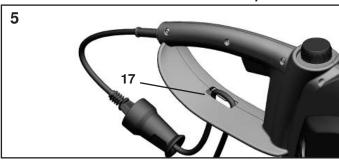
This chainsaw is fitted with a strain-relief device to provide extra safety for the connection. First connect the device plug with the connection line. Then form the connection line into a tight loop and push this through the safety web on the lower side of the machine. Hang the loop into the hook as shown in Fig. The plug connection is now secure against automatic release.
