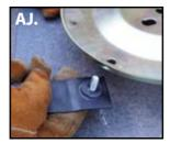
**NOTE:** There is 1 washer located under the screw on the outer side of the blade mounting plate (37), and one on the underside of the blade mounting plate in between the blade and blade mounting plate (37). Be careful not to lose these.
