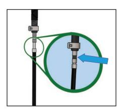
Use your free hand to grip the short section of pole visible below the handle (see the arrow shown above) and pull it downward.
