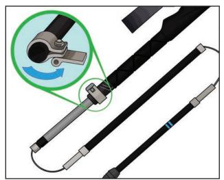
Open the white flick-lock lever on the handle, slide the top of the lower sections inside (the area with the height adjustment markings), then close the white flick-lock lever to secure the lower sections to the handle. You can then follow the normal assembly process on Page 1.
