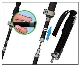
To collapse the pole for storage, simply depress the locking button to release it and push that upper section of pole back into the handle. This will loosen the rest of the pole which can be then folded for storage.
