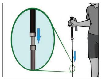
Hold the handle in one hand and let the rest of the pole hang free. Use your free hand to slide the loose middle section down to rest on top of the bottom section (see inset).
