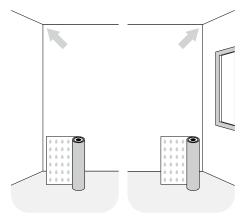
A wall covered with paint should be primed once, and in the case of a thick layer of paint (e.g. silicone, washable), rub with sandpaper (to increase the adhesion of the adhesive to the substrate) and degrease.
