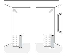
you can measure and draw vertical lines on the wall approx. 2 cm narrower than the width of the wallpaper or use a laser level.
