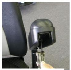
1. Raise arm and locate screw closest to end of armrest. Remove screw using an Allen Wrench
