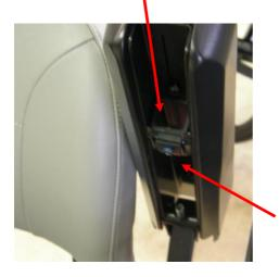
3. Insert Snaplt!™ mounting arm into receptacle with clip facing up.
