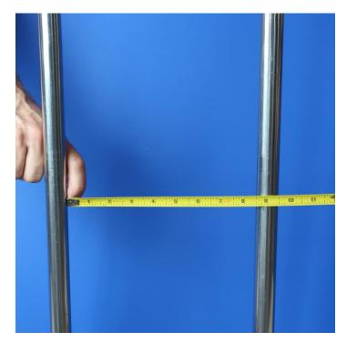
accurately to ensure that the guard fits properly and performs its intended function. As illustrated in the photo above you can see that the center-to-center spacing of this pedestal guard is 9 ½".
