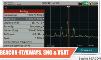
signals can be clearly seen thanks to the 1 MHz SPAN and 10 kHz
