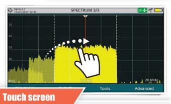
Place the marker on any channel and move the trace using your finger.
