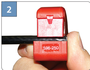
2 Using a fixed blade prep tool in good condition, prepare cable to 1/4" x 1/4" dimensions. Use edge of tool if no stop.
