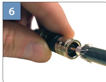
6 Guide center conductor and dielectric into post. Insert cable into connector until dielectric is flush within post.
