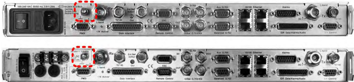
(TOP) Standard AC Chassis (CEFD P/N PL-0021325) (BOTTOM) Optional 48V DC Chassis (CEFD P/N PL-0021327) Figure 3-8. CDM-625A Chassis Ground Interface
