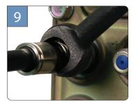
Tighten connector to recommended torque.
