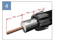
Cable is prepared to proper dimensions.
