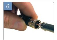
Guide center conductor and dielectric into post. Insert cable into connector until dielectric is flush within post.
