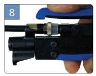
Using your VT-200 compression tool, make sure the rotating compression head is positioned for 6/59 as shown in the picture. Porperly seat connector and compress fully.
