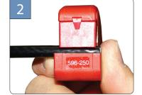
Using a fixed blade, prep tool in good condition, prepare cable to 1/4" x 1/4" dimensions. Use edge of tool if no stop
