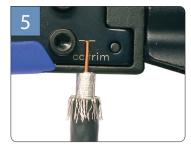
Ensure cable is prepared to 1/4" x 1/4" dimensions. Use guage on VT tool to recheck center conductor.
