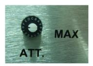
Using a screwdriver, turn the rotary switch to the required attenuation, according to the table below:-
