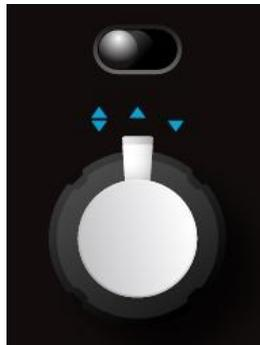
*Note the blue arrow markings above all attenuverter switches. The left-most 'up and down' arrows mark -1 to +1 range of the knob with the 12 o'clock position being 0. The center 'up' arrow marks 0 to +1 positive unipolar range. The right 'down' arrow marks 0 to -1 negative unipolar range.*
