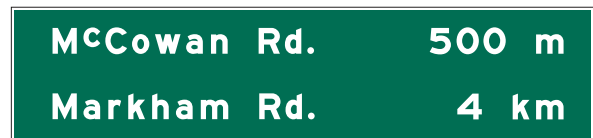
Figure 5.13: G112 – Freeway Interchange Sequence Sign
