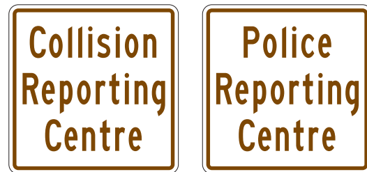
Figure 11.8: M405 – Collision/Police Reporting Centre Marker
