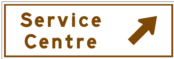
Figure 13.3: G406 – Freeway Service Centre Turn-Off Sign
