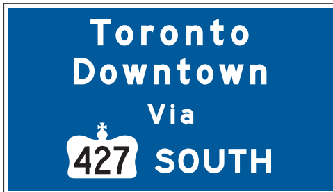
Figure 5.24: G323 – To Downtown or City Centre from Airport Sign
