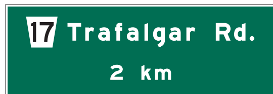
(a) G103 – Freeway Pre-Advance Sign
