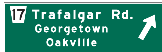
Figure 5.2: G101 – Freeway Turn-Off Sign (Ground-Mounted)
