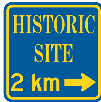
(c) G609 – Historic Site Route Marker
