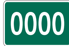
Figure 11.3: G218 – Emergency Services Property Identification Marker
