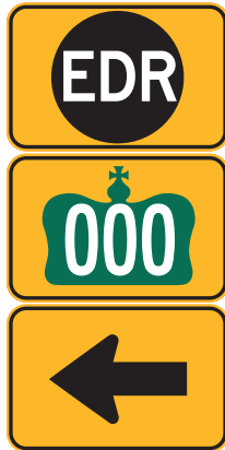
Figure 10.2: Sample of EDR Trailblazer OPEN sign assembly
