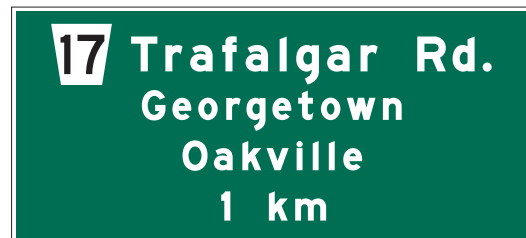
Figure 5.4: G100 – Freeway Advance Sign (Ground-Mounted)
