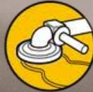
Spread out compound and polish at 1200-2000 rpm
