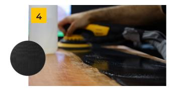
Wet sanding. Attach a vacuum block disc to the Deros before attaching the Abralon to protect the dust extractor and sander
