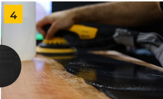
Wet sanding. Attach a vacuum block disc to the Deros before attaching the Abralon to protect the dust extractor and sander
