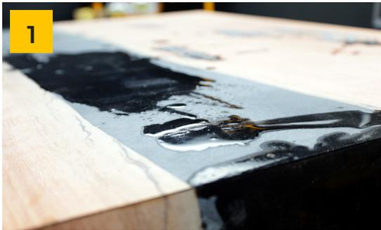
Using the Mirka Deros Sander, sand the epoxy with Abranet Ace HD 40 grit to remove excess resin
