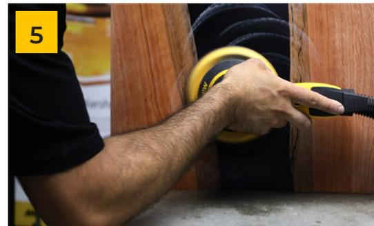
Wet sand the epoxy surface with Abralon using water in higher grits to make the epoxy surface smooth, 360, 600, 1000, 2000, and 4000 grit.
