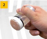
Always use water when sanding, apply water to both abrasive and the defected area. Use Mirka damper for best result.
