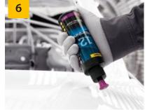
Apply a small amount of Polarshine® 12 on the polishing pad or directly to the defected surface area.
