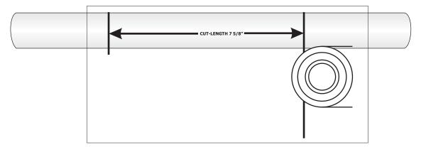
Fig. A - Determine plumbing size
