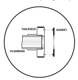
**9 -** You are now ready to install the heater in the open space between the two (2) tailpieces (ensure that the gaskets remain in place). Slide both heater nuts inward toward the center of the heater to expose the mating surfaces of the heater housing. Slide the heater carefully into place between the tailpieces and gaskets and hand-tighten heater nuts. If you use a wrench be careful not to over-tighten, the nuts can crack.
