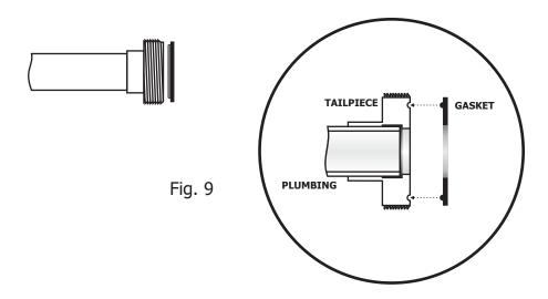
**4 -** You are now ready to install the heater in the open space where the Heater Ready fitting was located (ensure that the gaskets remain in place). Slide both heater nuts inward toward the center of the heater to expose the mating surfaces of the heater housing. Slide the heater carefully into place between the tailpieces and gaskets and hand-tighten heater nuts. If you use a wrench be careful not to over-tighten, the nuts can crack.
