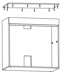
•Insert twelve (12) Camlock Screws into the Top Panel.
