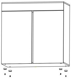
Step 10- Installing the cabinet **feet** [requires four [4] cabinet feet and four (4) 1" cabinet feet screws]
