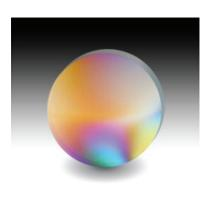
When viewed under a polariscope, optics with high stress will exhibit a distinct pattern as the light travels through it.
