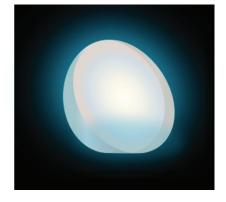
Some optical materials, when exposed to high energy UV radiation, absorb and re-emit the energy as light.
