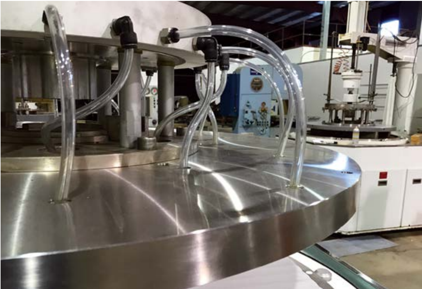
A bank of Speed Fam 16 B double sided polishers ready for service in Esco's new facility.
