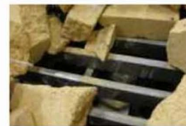
Cast iron grating with brick pieces for even heat distribution
