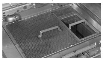
**Soil Management System.** Screen design sheds soil more easily than flat screens, reduces frequency of cleaning — easy to empty large soil particles . . . Just lift out the scrap basket.
