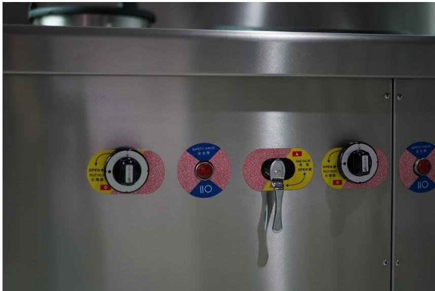
From left to right: Pilot flame valve(black), flame failure device(safety valve, red), main gas open valve (silver)
