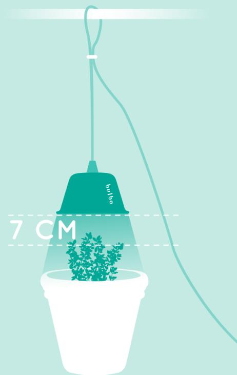
In order to shorten the cable and distance the Cynara from the leaves, disconnect blocker **E** and let the cable slide downwards.
