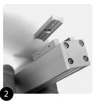
Move sliders on MoMo-L base to match plate spacing. Lock slider in position (grub screw/hex key).
