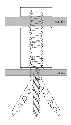
Use the holes in your material as a template to mark holes on your mounting surface.
