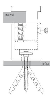
Mount the grippers to your panel by placing the grippers on the edges and tightening the nylon tips against back of the panel.
